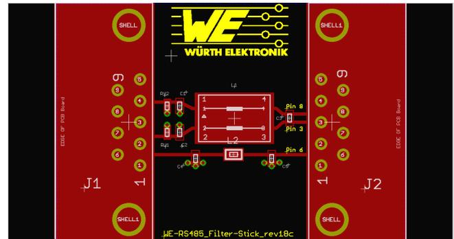
Figure 16: Complete filter stick design.
